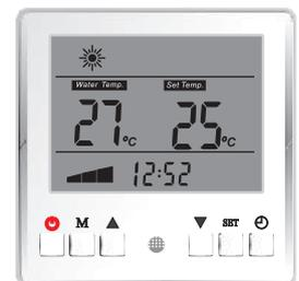
Picture shows that heating and hot water mode is selected
