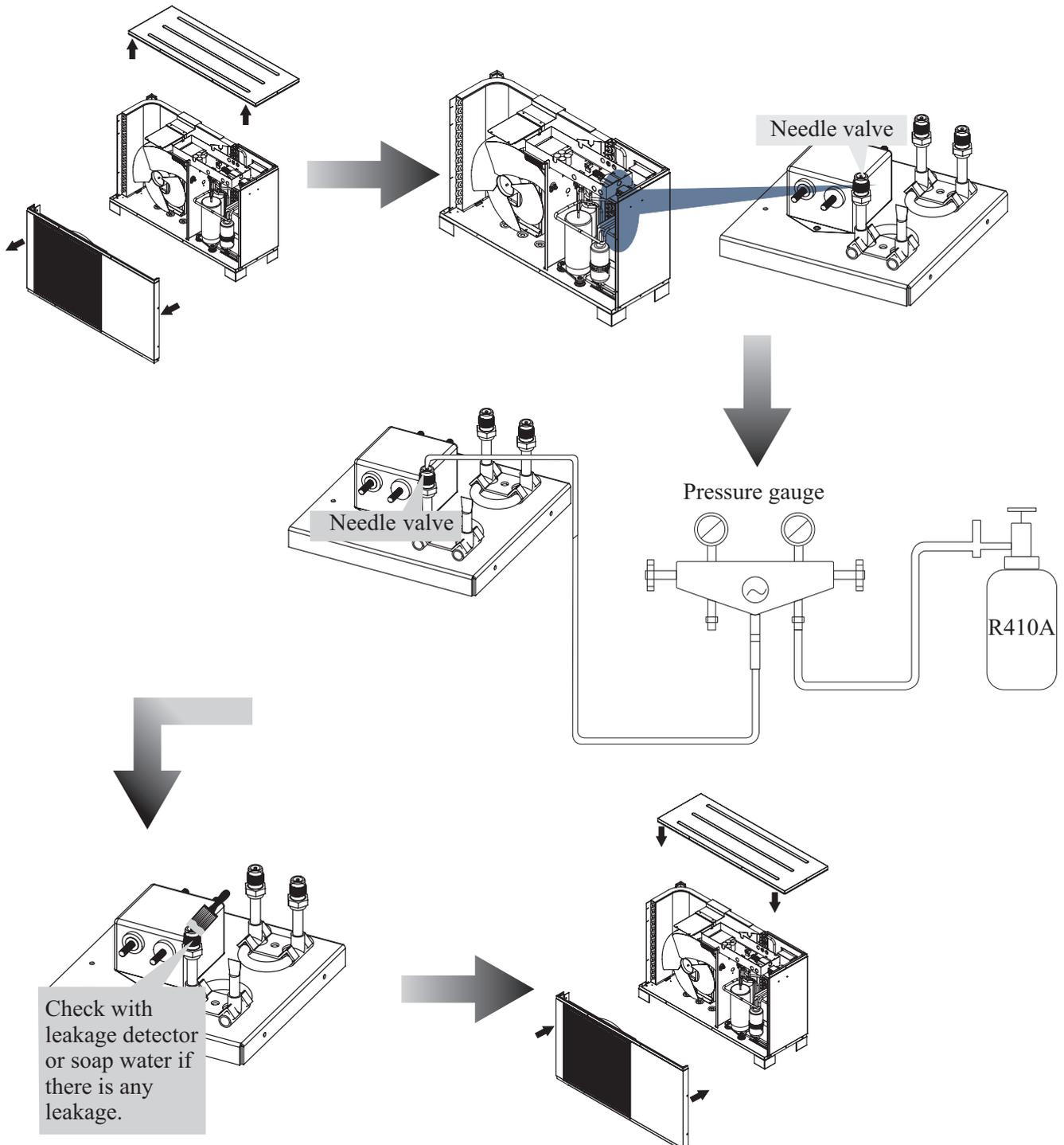
**Note:** Always use a weight scale to measure the gas amount charged into the unit.
