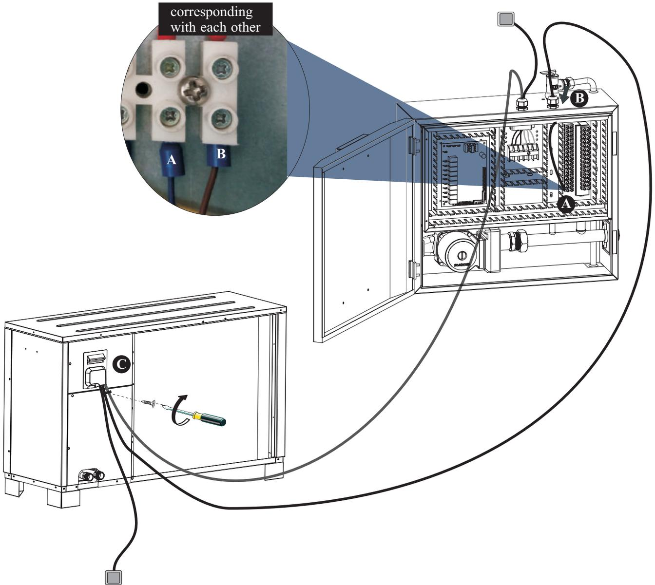
A. Insert one end of this cable through the cable gland on top of the indoor control unit, and connect this cable to A, B, on terminal block.
