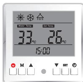
Press ▲ and ▼ for 5 seconds in main interface, to activate inquiry of current running status.
