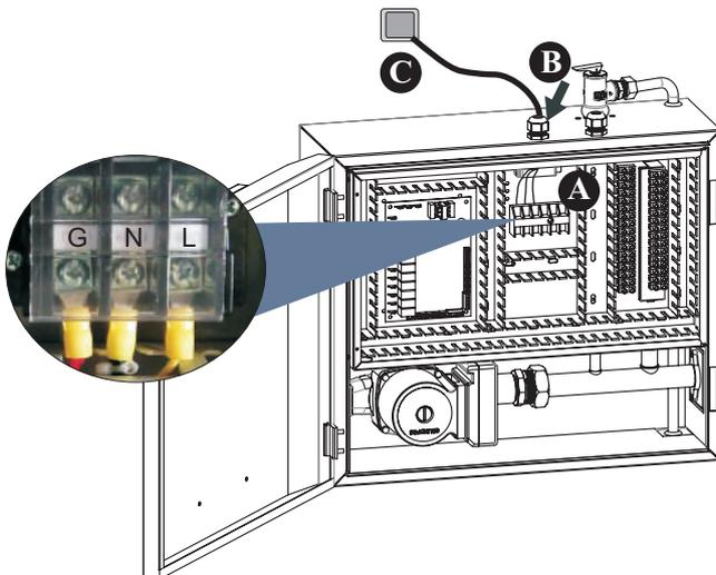
A. Insert one end of this cable through the cable gland on bottom of the indoor control unit, and connect it with heat pump power supply terminals (G, N, L).
