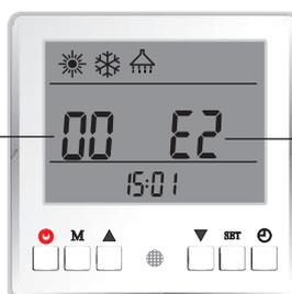
Failure code or protection code
