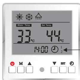
This symbol means the unit is in sanitary hot water and cooling/heating Timer ON period. Unit will work for both hot water and cooling/heating mode (not in same time) when needed.
