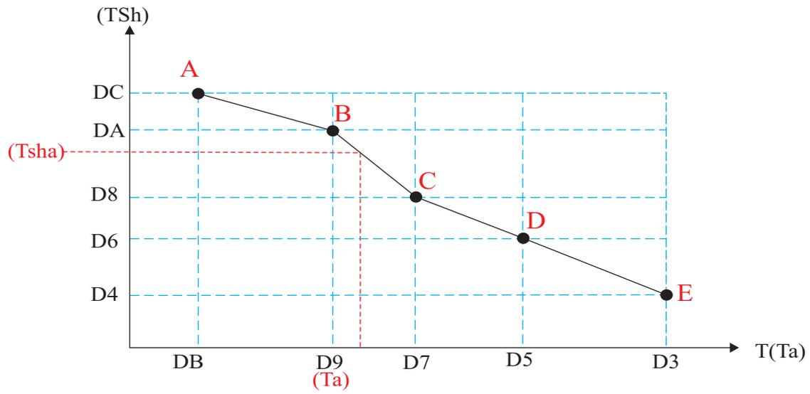
As shown here, actual set water temperature (TSh<sub>a</sub>) is calculated according to actual ambient temperature (T<sub>a</sub>), according to this created curve.
