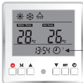
This symbol means the unit is in sanitary hot water Timer ON period. Unit will work in hot water mode when needed.
